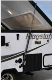
Power Roof Lift Assist (Std. T19QBHW, T19SCHW, T21QBHW, T21TBHW, T21DMHW Only)
